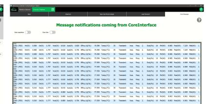
Load Transient PWM Configuration Tab Control over Frequency, PWM positive duty cycle, normal operation/load transient and measurements of input/output power, output voltage/current
