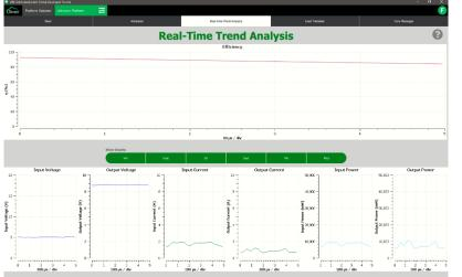
**Real-Time Trend Analysis Tab** Efficiency, input/output voltage, input/output current, input/output power graphs
